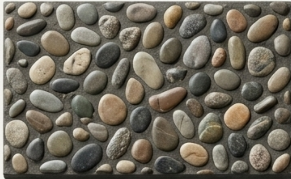
Exposed Aggregate: River Stone
